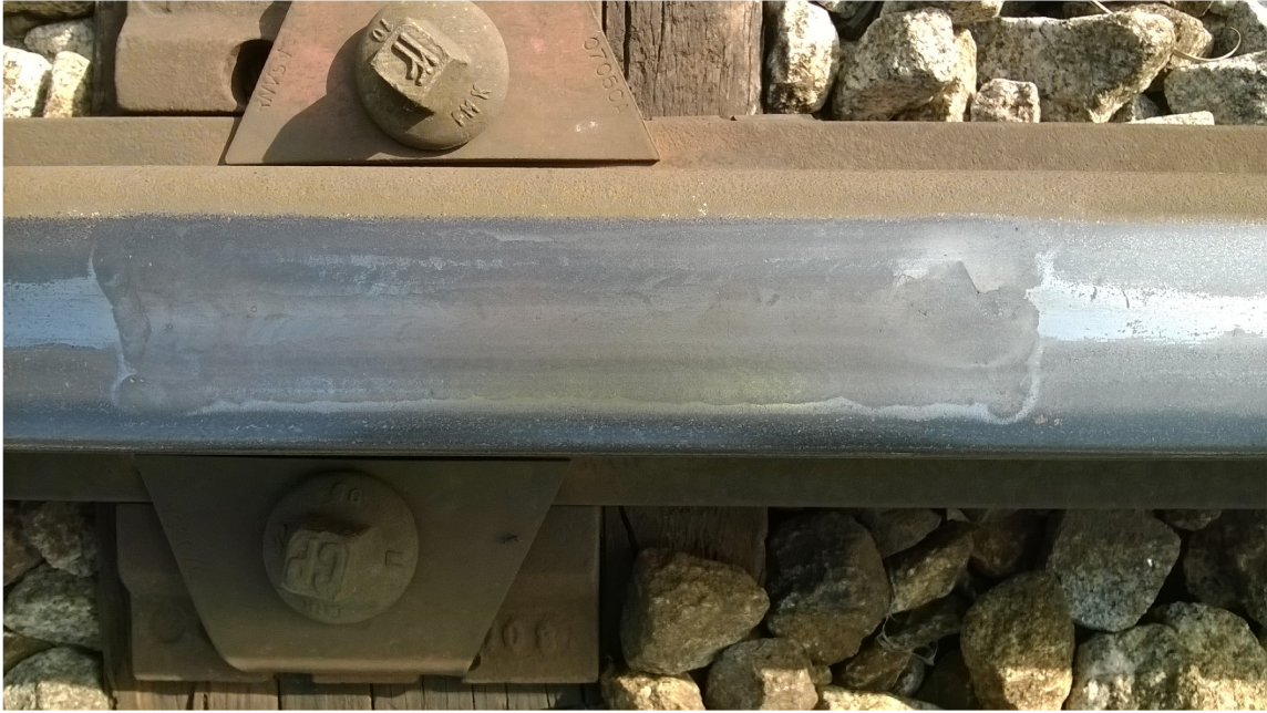
Figure 2 — Porosity on electric arc repair welds (b)
