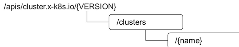
Figure 6.3-1: Resource URI structure of Cluster resource object for the CIS cluster lifecycle management service interface
