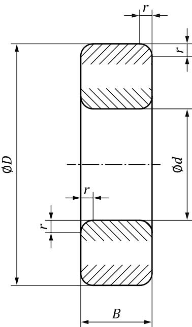
**Key** $B$  bearing width $D$  bearing outside diameter $d$  bearing bore diameter $r$  chamfer dimension $r_{s \min}$  smallest permissible single chamfer dimension
