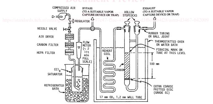
Note 1—These items for the apparatus are critical: the dimensions of the sample tube; the location of the flowmeter downstream of the  $CCl_4$  saturator; and the location of the stopcocks. Reheat coil must be adequate to bring the gas temperature to within 1°C of the water bath temperature (that is, bed temperature).
