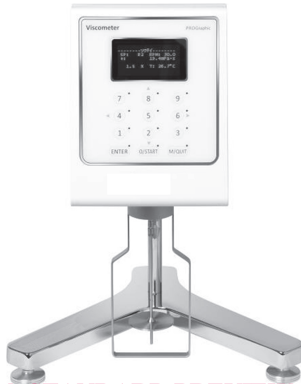
Figure 3 — Example of single cylinder type rotational viscometer for model R, H(A) and H(B)
