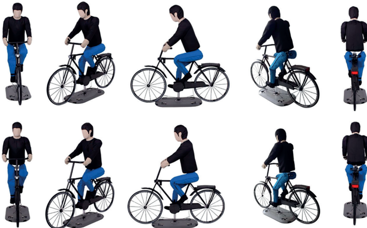
iTeh STANDARD PREVIEW Figure 1 — Bicyclist target with different BT rider torso angles (standards.iteh.ai)
