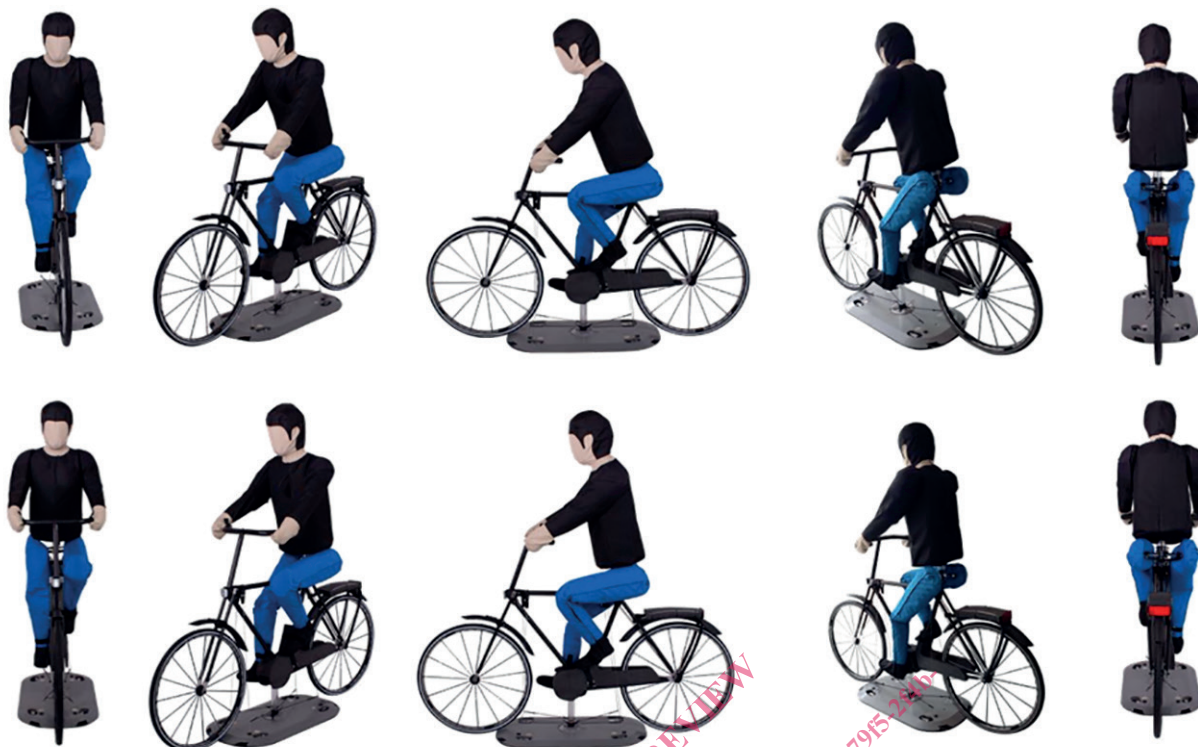
Figure 1 — Bicyclist target with different BT rider torso angles
