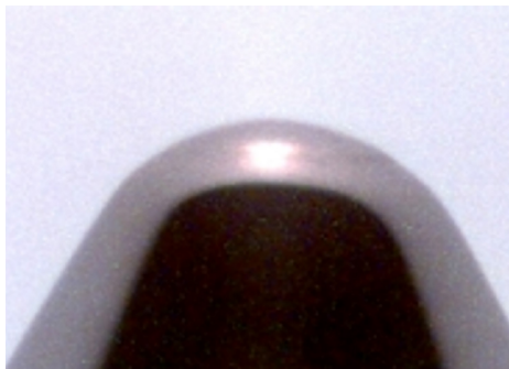
Figure 2 — Correct shape of the scratching tip
