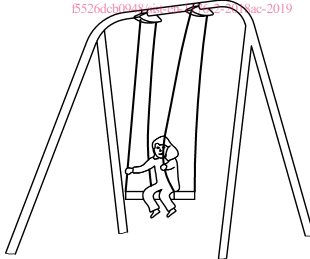
Figure 2 — Example of a swing with several rotational axes (Type 2)
