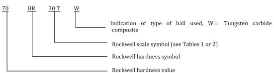
NOTE 1 Previous versions of this part of ISO 6508 allowed the use of steel indenter balls, which required the suffix S.
