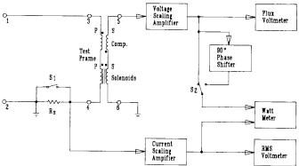
FIG. 1 Basic Circuit for Wattmeter-Varmeter Method
