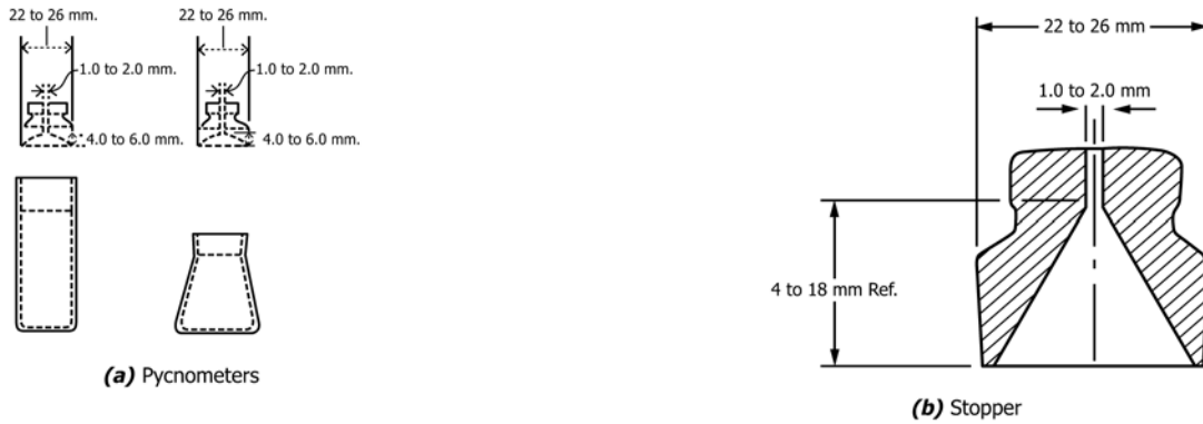
FIG. 1 Suitable Pycnometers and Stopper
