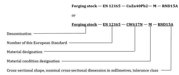
EXAMPLE 2 Forging stock conforming to this standard, in material designated either CuZn40Pb2 or CW617N, for drinking water applications according to the 4 MS Common Composition List, in material condition M, round, nominal diameter 15 mm, tolerance class A, will be designated as follows:
