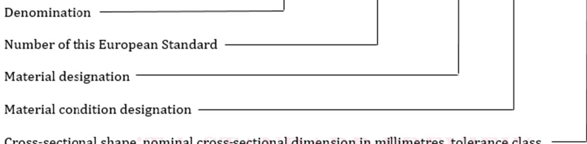
**EXAMPLE 2** Forging stock conforming to this standard, in material designated either CuZn40Pb2 or CW617N, for drinking water applications according to the 4 MS Common Composition List, in material condition M, round, nominal diameter 15 mm, tolerance class A, will be designated as follows:
