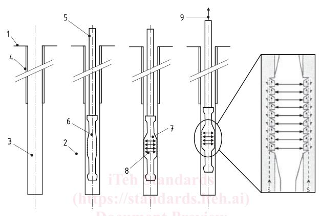
a) Borehole drilling phase: drilling a phicometer borehole with casing (if necessary) and setting up the PBST test pocket in the borehole bottom
