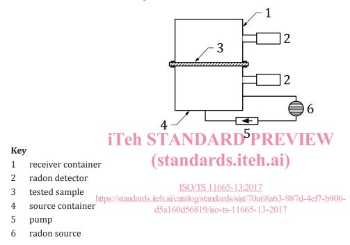
Figure 1 — Measuring system comprising one receiver container and one source container
