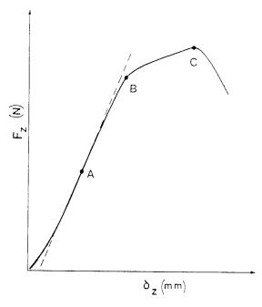
Note—Stiffness is defined as the slope of the linear-most portion of the curve, here evaluated by a tangent drawn at Point A. Point B illustrates a slope discontinuity (possibly indicative of interfacial slip or subcomponent failure within the connector), and Point C illustrates the maximal load acceptance (ultimate strength).
