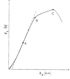
Note—Stiffness is defined as the slope of the linear-most portion of the curve, here evaluated by a tangent drawn at Point A. Point B illustrates a slope discontinuity (possibly indicative of interfacial slip or subcomponent failure within the connector), and Point C illustrates the maximal load acceptance (ultimate strength).
