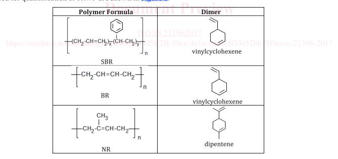
Figure 1 — Dimeric pyrolysis products of tyre rubber polymers
