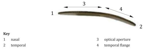
Figure 1 — View from above of an example of a right lens with a temporal flange
