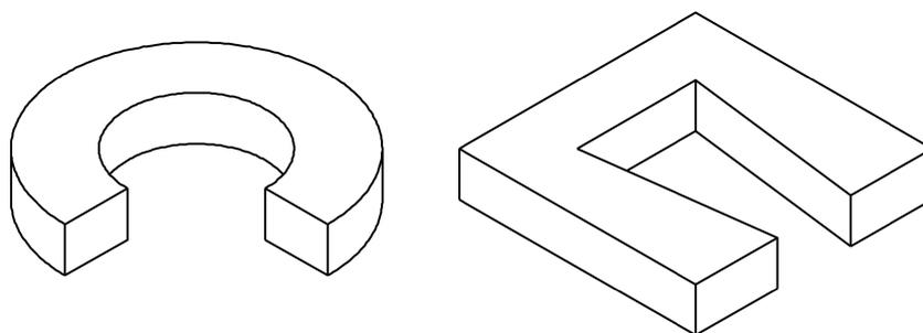
**Figure 3 — Examples of partially bound openings**
