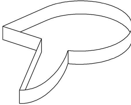
**Figure 5 — Example of an irregular shaped opening**
