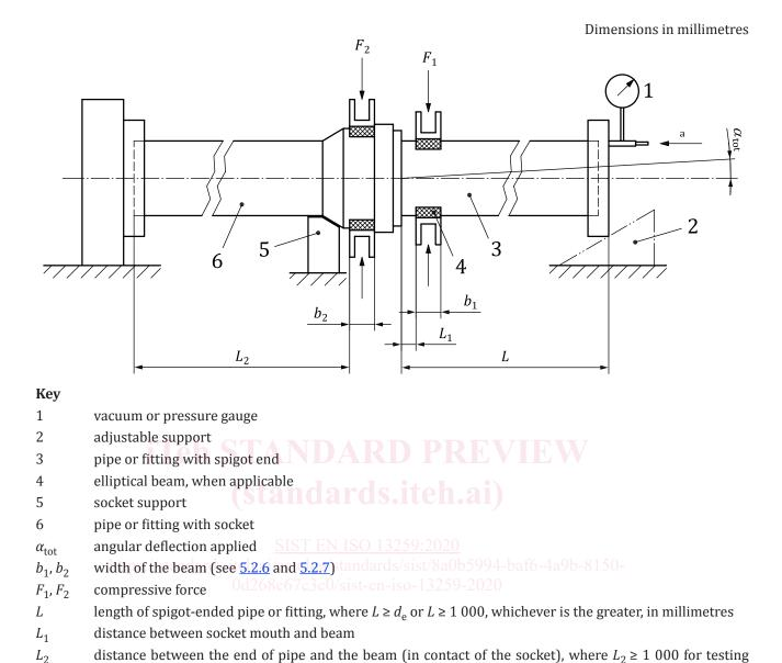
Figure 1 — Typical arrangement for applying diametric deflection and angular deflection
