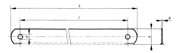
Blade length I is the distance between centres of pin holes. It is recommended that the centre of the pin hole be located on the centreline of the blade.
