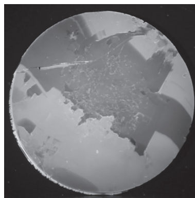
Figure 1 — Crystal grains in UVPL image (clear lines of grain boundary expressing crystal shapes)
