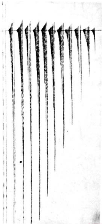
FIG. 12 Sample Drum Record of Impact Bending Test
