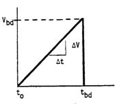
FIG. 1 Voltage Profile of the Short-Time Test
