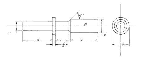
A = minimum expanded diameter of tubing as supplied.
