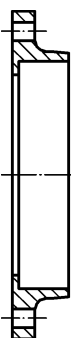
Type 14 Hubbed slip-on flange in copper alloy supplied with tube stops, for soft soldering, brazing or welding
