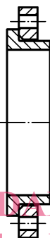
Type 07, 37 Loose plate flange in steel with a slip-on collar (type 37) in copper alloy for soft soldering, brazing or welding
