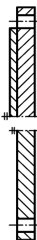
Type 05, 05C 05 Blank flange in copper alloy 05C Blank flange in steel clad with a copper alloy jointing face
