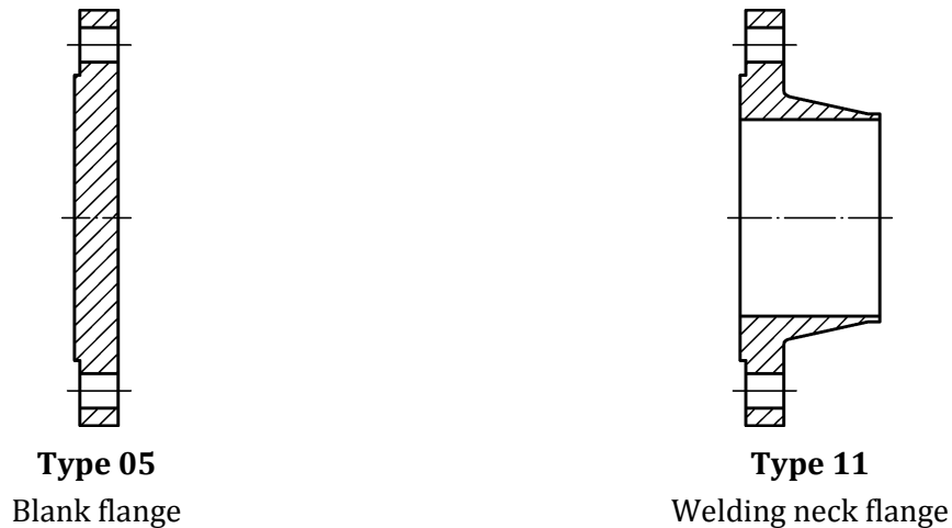
Figure 1 — Types of flanges
