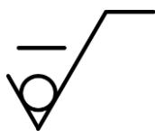
Figure 4 — Graphical symbol indicating profile surface texture
