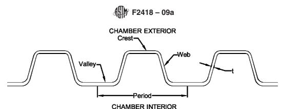
Note—The corrugation profile shown in this standard is intended only as a general illustration. Any corrugation pattern is permitted, as long as it meets all the specified test requirements of this standard.
