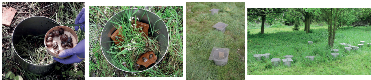
Figure 1 — In situ exposure: Active biomonitoring using microcosms where snails are exposed (from left to right: sub-adult snail, total fresh mass 4 g to 6 g); open microcosm; microcosms covered by a stainless steel netting (mesh size: 10 mm) securely fitted over the top of the microcosm by 4 pickets; microcosms on site)
