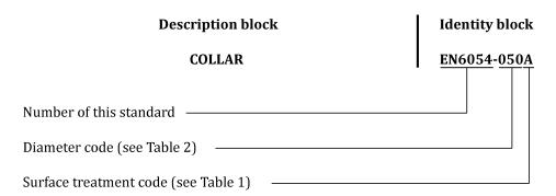
If necessary, the code I9005 shall be placed between the description block and the identity block. Example of part numbering in accordance with ATA iSpec 2200 (15 character rule).
