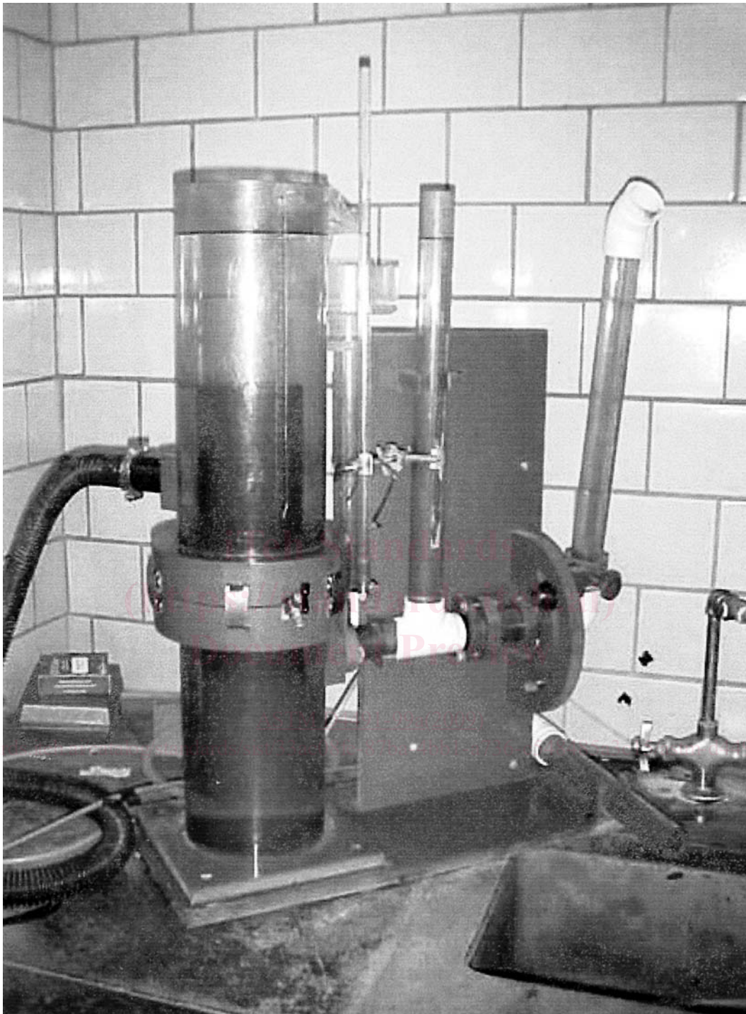
FIG. 1 Constant and Falling Head Permeability Apparatus
