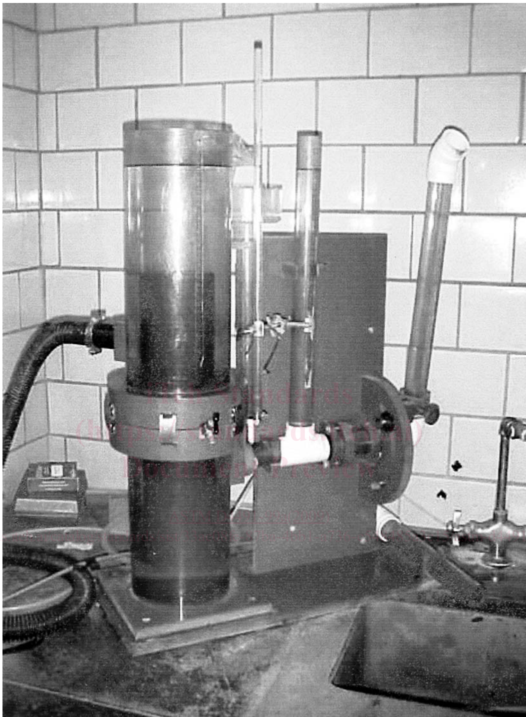
FIG. 1 Constant and Falling Head Permeability Apparatus
