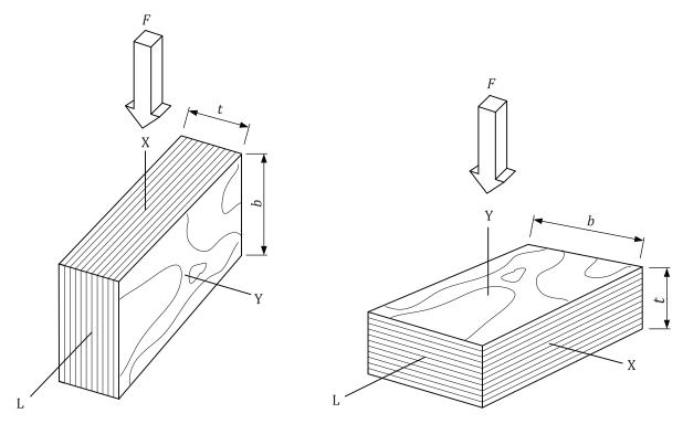
a) Cross-section related to edgewise (Joist) bending b) Cross-section related to flatwise (Plank) bending
