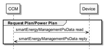
Figure 2 — Example communication sequence diagram
