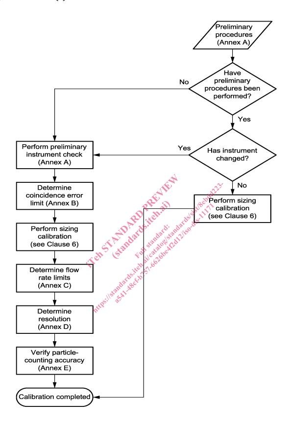
Figure 1 — Recommended sequence of APC calibration procedures
