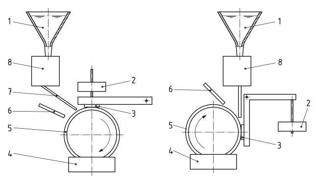
a) With horizontal test piece
