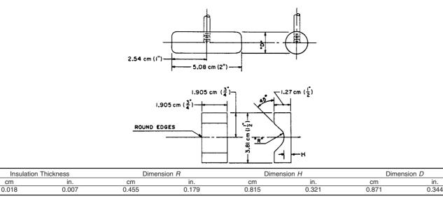
Tolerance for R and D = 0.003 cm (0.001 in.) Tolerance for H = 0.005 cm (0.002 in.)
