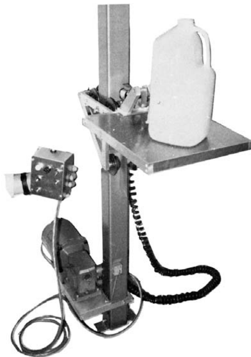
FIG. 1 Apparatus for Dropping Containers
