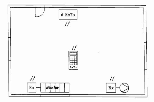
Figure 3: Heating, ventilation and air-conditioning control
