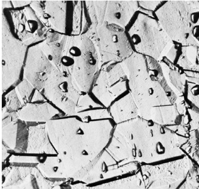
FIG.-2_1 Step Structure (500×) (Steps between grains, no ditches at grain boundaries)
