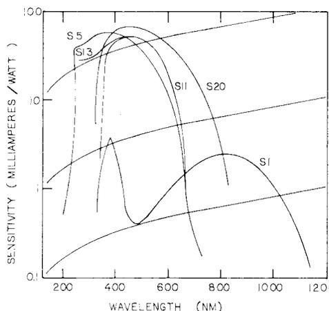
**FIG. 3 Spectral Response Curves for Several Cathode Types**
