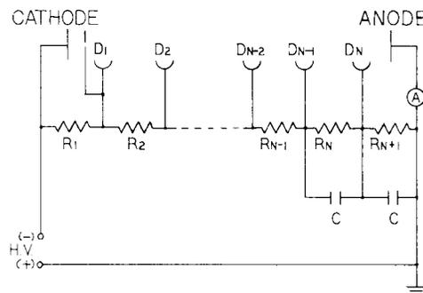
**FIG. 4 Voltage-Divider Bridge**
