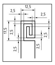
NOTE The wire diameter is usually 0,1 mm to 0,3 mm.
