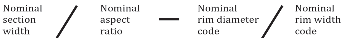
Figure 1 — — Indication of dimensional and constructional characteristics
