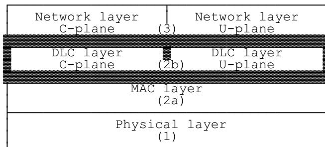
Two planes of operation are specified for this data link control (sub)layer. These planes are called the C-plane (Control plane) and the U-plane (User plane).
