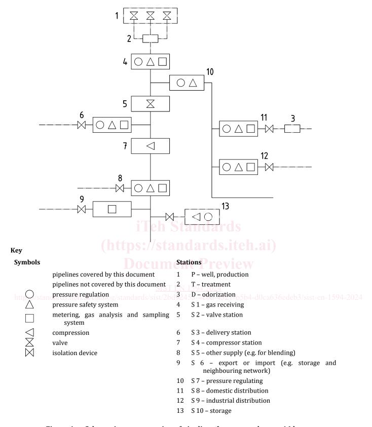
Figure 1 — Schematic representation of pipelines for gas supply over 16 bar
