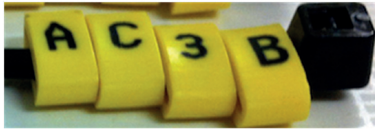
Figure 2 — Code identifying that the sample is attached with a cable tie to the frame
