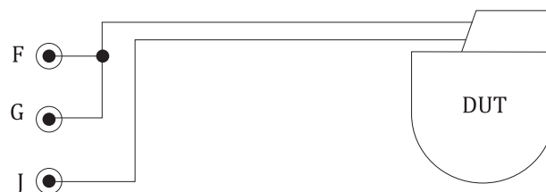
Figure 6 — Differential mode connection to single-channel bipolar device
